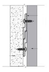
This is a typical Z-clip that is used for the wall attachments
